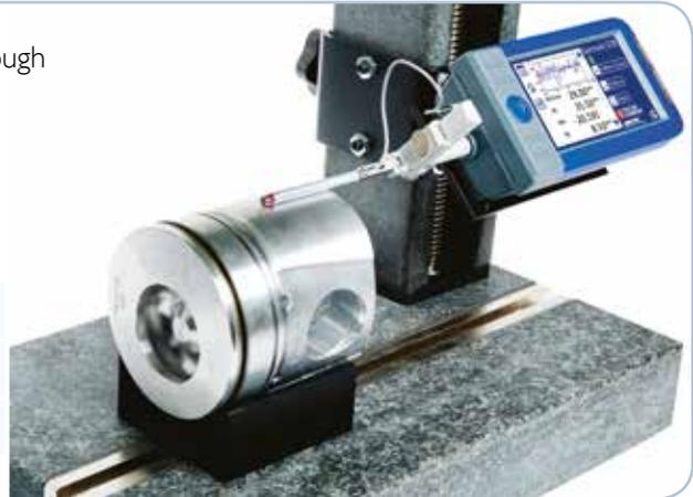
**Intra Touch / Intra Contour** are a range of precision shop floor solutions for surface finish and contour measurement.
