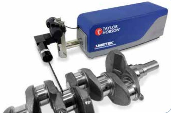
**Surtronic® R-100 Series** robust enough for the shop floor but accurate for any inspection area, giving a flexible solution for all roundness and form measurements. Improved feature set includes advanced harmonic analysis and higher gauge resolution.
