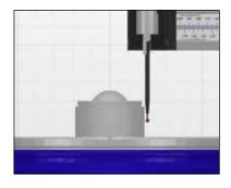
A simple approach to gauge calibration that literally takes seconds to do. Utilising the instrument high precision scales this procedure calibrates both the gauge gain and crutch angle position in a single user guided
