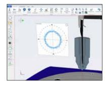
A powerful utility that enables online and offline programming around a CAD model. Features include a stylus tip "flight path" enabling collision detection.
