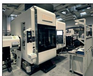
Taylor Hobson's latest investment includes the Mazak Integrex i-200S with 10 axis, twin spindle, in cycle probing, tool break detection, unmanned running, temperature control, zero set up times, auto re-loading, high accuracy glass scales and 110 tool capacity.
