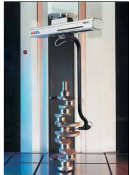
Complex crankshaft measurements can be performed automatically with the crankshaft accessory arm and powerful analysis software
