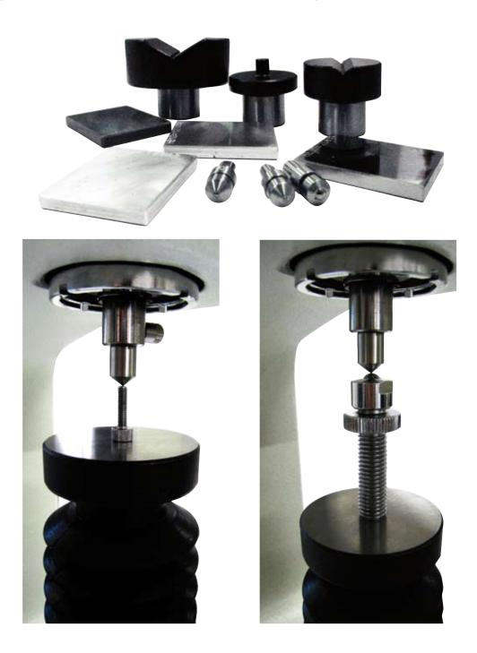
The NR3D hardness tester has a diversified application field. With the different available combinations of standard loads and indenters, it is possible to test very hard materials as well as soft and plastic ones, of different shapes and dimensions.
