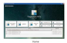
or statistical analysis are standard functions. The software consists of two parts: the "Testing" and "Data Processing" components. Since both software components can be opened simultaneously, data can be processed while tests are being performed, allowing testing to be executed efficiently.
