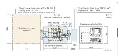
Note: The main unit of the testing machine must be installed on the first floor of a building, on a concrete floor that has a thickness of at least 250 mm (capable of withstanding the own weight of 1,500 kg). The foundation needs to be constructed by the user. Avoid installing the machine on an upper or hollow floor, due to the impacts and vibration generated during high-speed testing.
