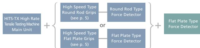
The grips, force detector (either for round rods or flat plates) are selected and combined with the main high-speed tensile testing machine.
