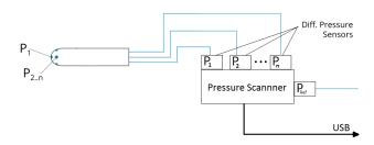
Figure 3: Multi-hole probe pressure tube connection
