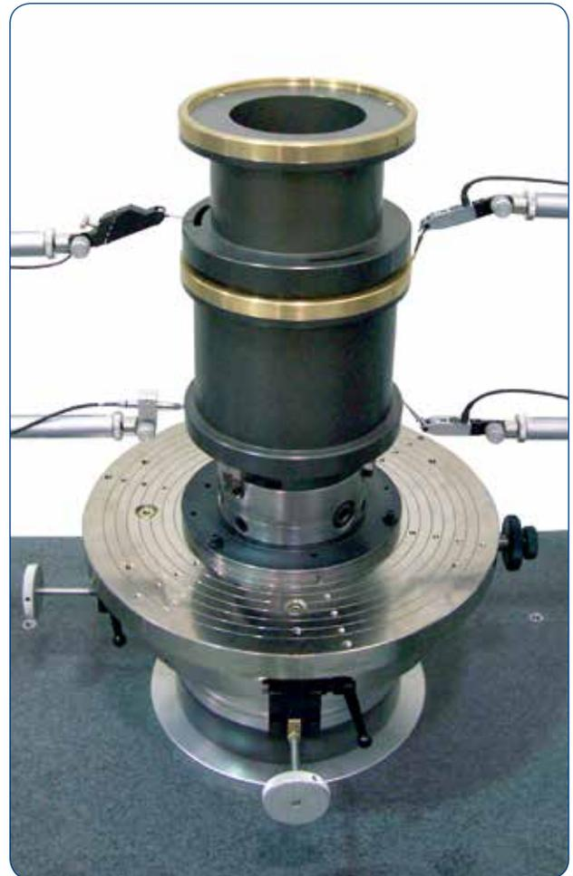
Multi-gauge measurement for component stacking
