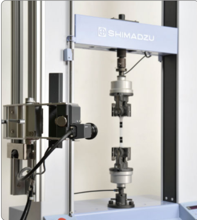
AGS-10KNXD + Pneumatic Flat Grips + TRViewX Non-Contact Digital Video Extensometer
