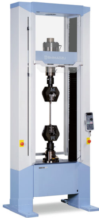
AGS-300kNX + 300kN Non-Shift Wedge Type Grips
