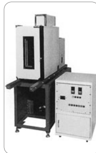
AGS-10kNXD + Screw Type Flat Grips + Compact Thermostatic Chamber TCE series
